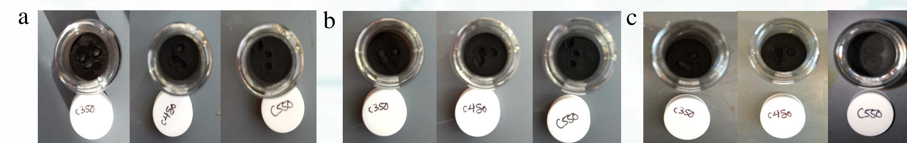
Figure 3. Water Droplet Penetration Test photos for Corn samples. a) After 1 minute; b) After 10 minutes; c) After 60 minutes. The C350 sample showed the highest degree of water repellency.
