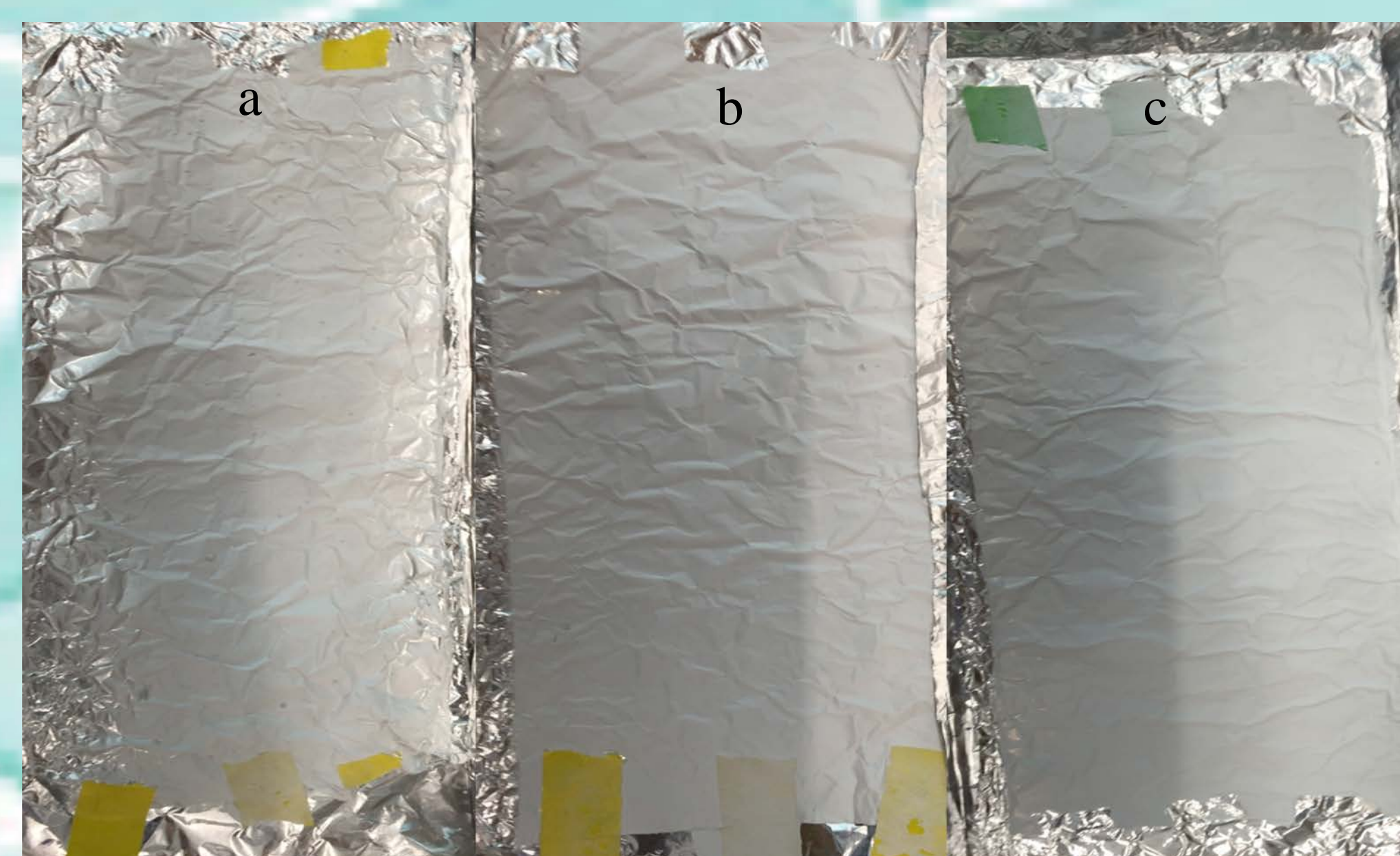
Figure 2. Electrospun membranes with W350 biochar. The membranes were spun with a) unsieved biochar; b) <10 μm biochar, c) no biochar for a control.
